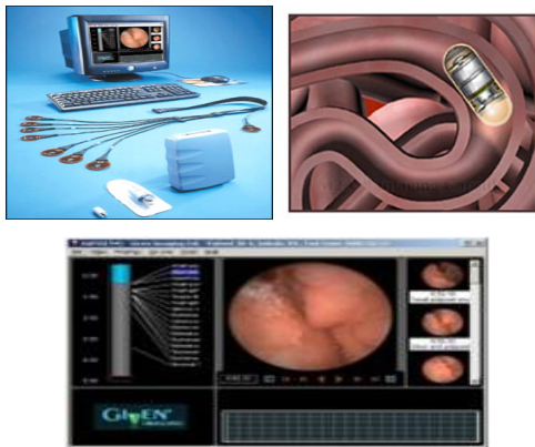
Figure 1: WCE system: (a) capsule and data recorder; (b) GI transit; (c) Rapid Reader from Given Imaging, Ltd.
